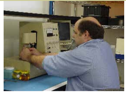
Jerry Green working with the Kester (KS-150) Solderability Tester
